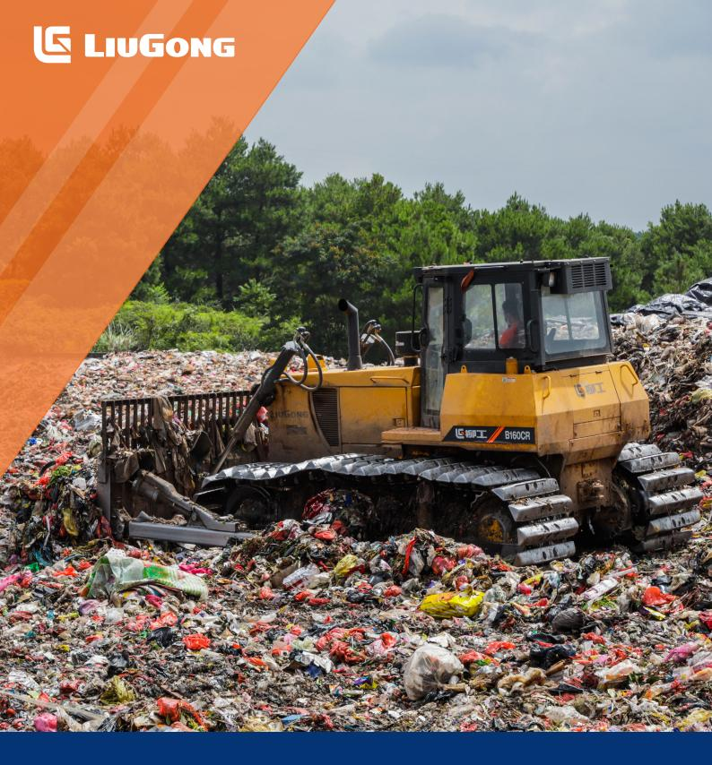
Engine Weichai WD10G178E25 Gross Power 131 kW (176 hp / 178 ps) @ 1,850 rpm Net Power 120 kW (161 hp / 163 ps) @ 1,850 rpm Maximum Torque 830 N  $\cdot$  m Blade Capacity 10.4 m³ Operating Weight
